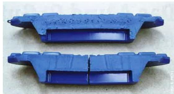
By using equal vulcanisation times, due to variothem temperature control the lower part of the cold runner nozzle is vulcanised, whereas the upper part at constant controlling is not yet fully cross linked.
