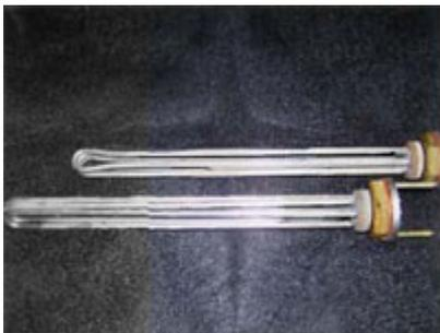
Before these two heat exchangers were covered with a thick glycol-crustification, now they have been cleaned.
