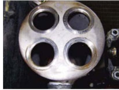
Cleaned heat-container filled with Inox Cleaner ®
