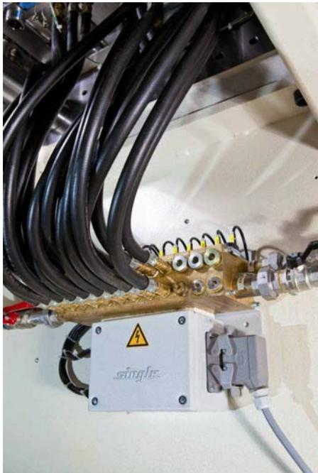
*SWV water distribution system for wear-resistant and precise flow metering and return temperature measurement operated on an injection moulding machine with particularly short mould connection tubes*
