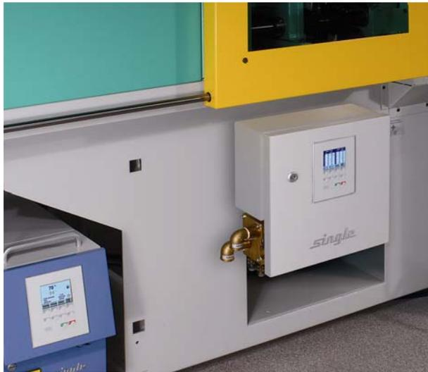
*The SWV water distribution system is ideal for wear-resistant, high-precision flow metering in injection moulding machines.*
